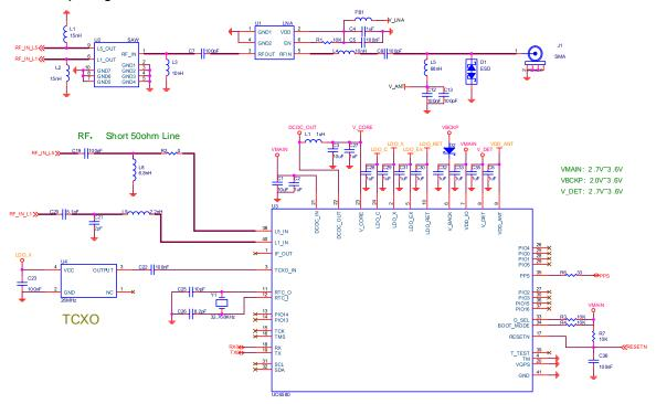
Figure 1-2 Reference design of DCDC mode
