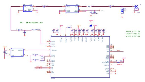
Figure 0-1 Simplest design to replace UC6226
