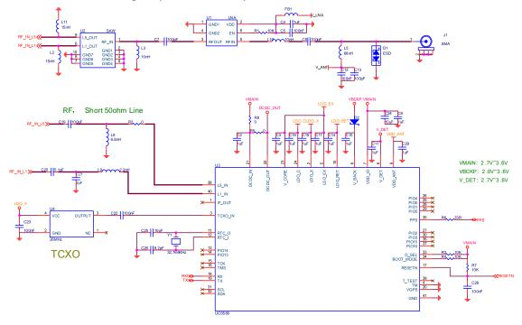
Figure 1-1 Reference design of LDO mode
